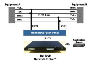
The Monitoring Patch Panel is a passive device. Each Monitoring Patch Panel consists of 32 female RJ45 connectors for the connection of E1/T1/J1 links to be monitored.
