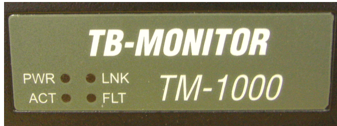
Figure 9 TM-1000 Front View LED description
