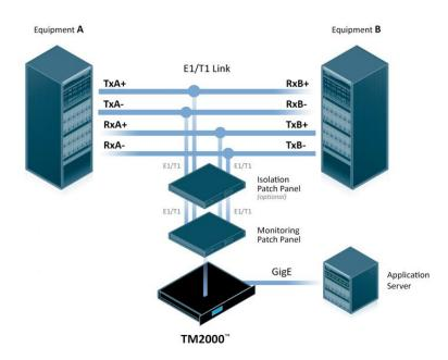
**Carrier-grade performance.** The *T*monitor TM2000 is a high volume monitoring solution. Multiple TM2000 devices and application servers can be clustered together in one or more facilities to provide essentially unlimited scalability. Application servers can also be deployed remotely for fully distributed monitoring.
