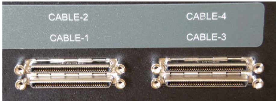
Figure 16 TM-1000 rear view SCSI-3 input connection
