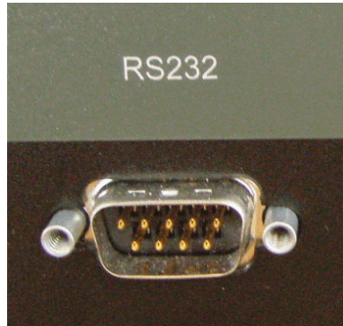
Figure 13 TM-1000 rear view RS-232 Link
