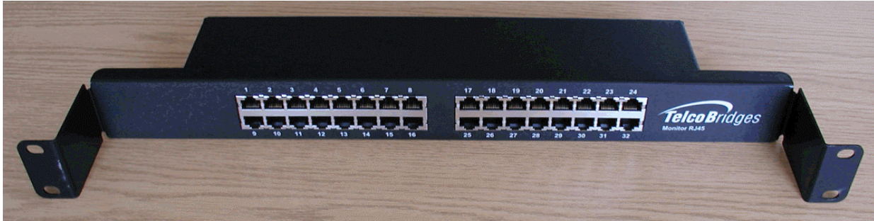
Figure 18 Patch panel front view
