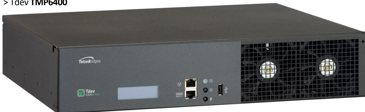
2U form factor with redundant power supplies shown here; a 1U unit with a single power supply is also available
