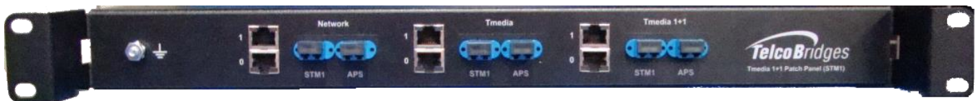
Tsig TSG3200-STM1 1+1, Patch Panel (front view)
