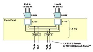
The Tapping Patch Panel is a passive device. Each Tapping Patch Panel consists of 32 female RJ45 connectors for the connection of up to 16 T1/E1 links to be monitored.
