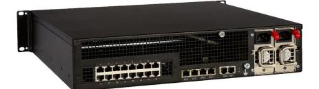
The TSG3200 is a high-capacity, 2U Signaling/SIGTRAN gateway and converter. The TSG3200-RJ can have from 8 to 16 T1/E1 ports. These ports are hardware ready, such that additional T1/E1 can be added via an easy software upgrade.
