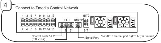
A) Connect to power sources B) Turn on power (if only one power source is used, press green button at rear of unit to disable the Power Power audible alarm). socket 1 3 5 7 9 11 13 15 Audible alarm button 1 2 3 RS232 BIT1 C) Verify Power LED = Solid Green (Refer to Panel 3)
